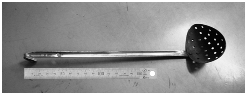
Figure 2 – Example of dross removal tool
