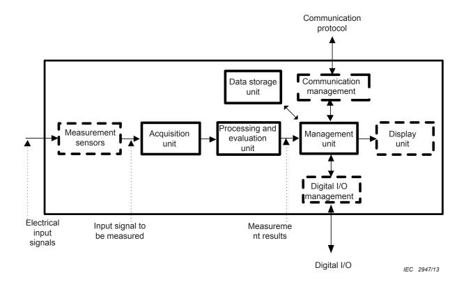
Figure 1 – Instrument generic measurement chain
