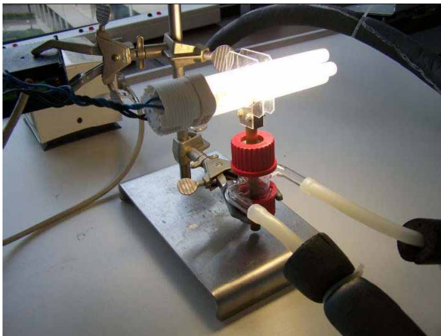
Figure B.2 – Example of cooling device arrangement
