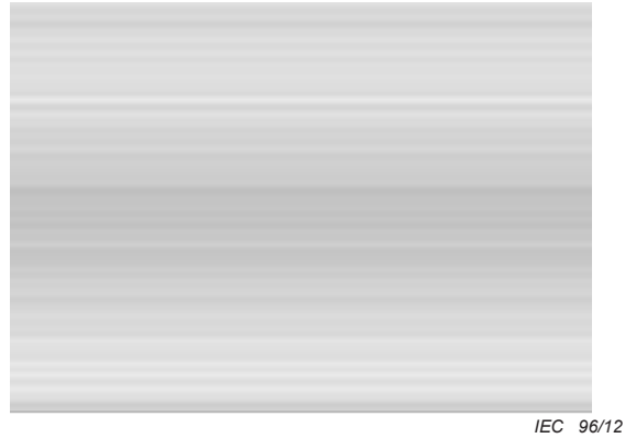
Figure 10 – Sample image of line mura defect associated with TFT non-uniformity
