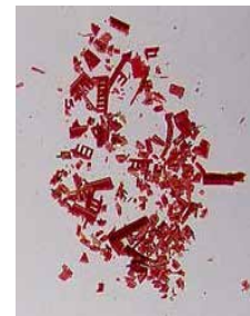
Figure E.9c – Integrated circuit lead frame package after disjointment
