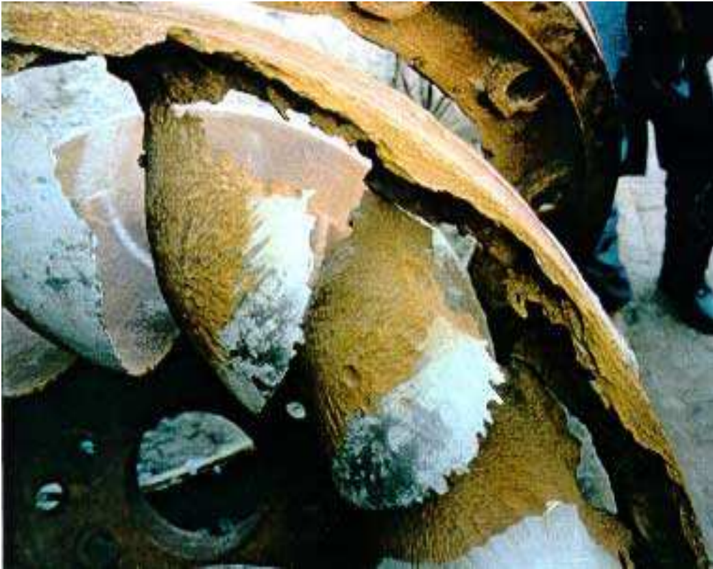
Figure 11 – Severe particle erosion damage in a Francis runner
