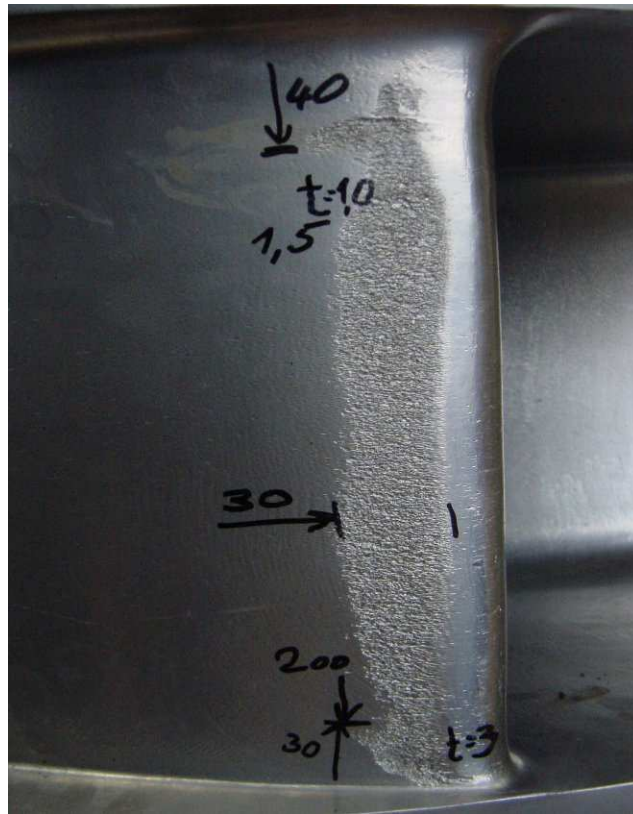
Figure 10 – Leading edge cavitation erosion on a Francis pump-turbine caused by extended periods of operation at very low loads
