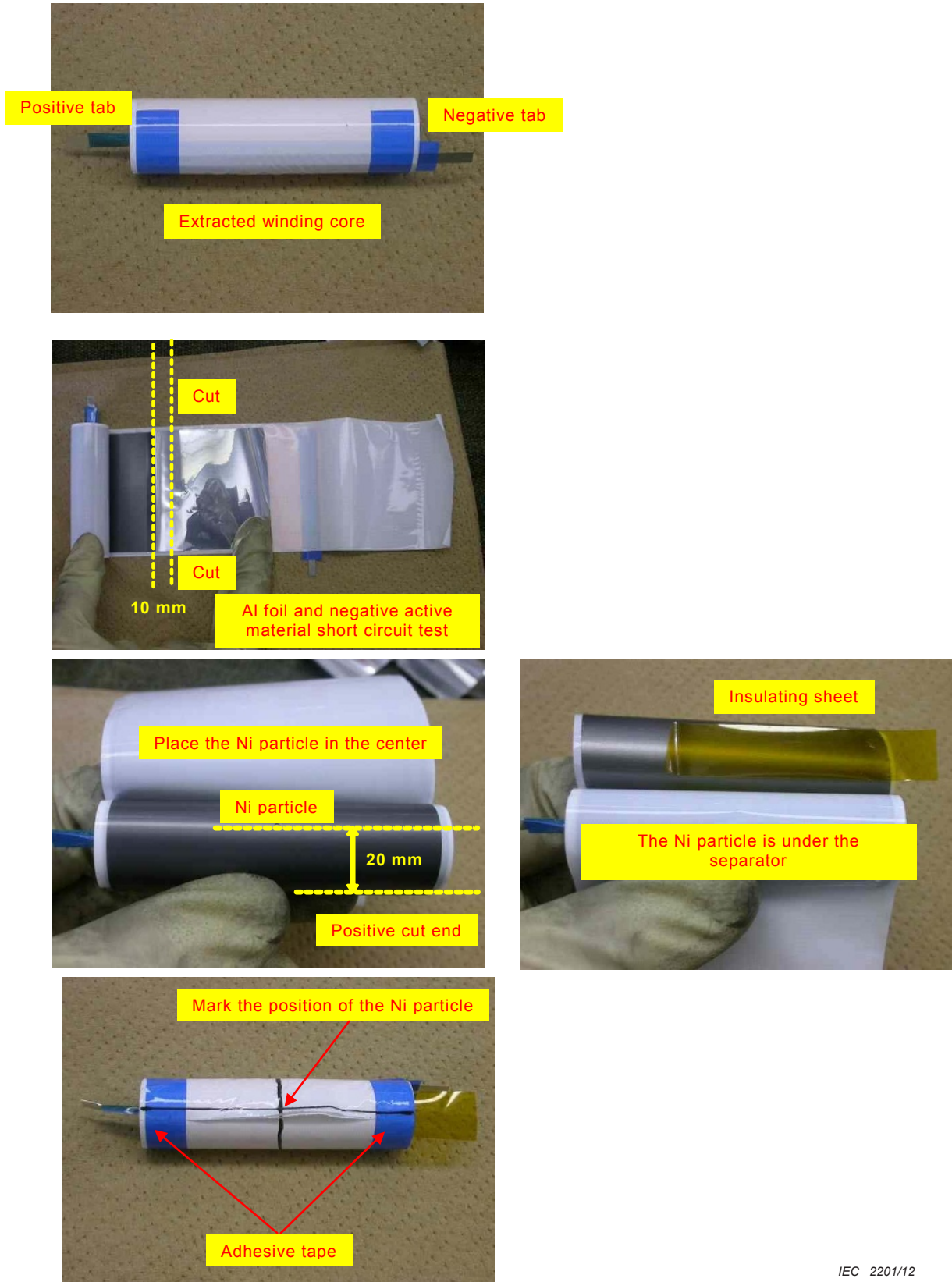
Figure A.5 – Disassembly of cylindrical cell
