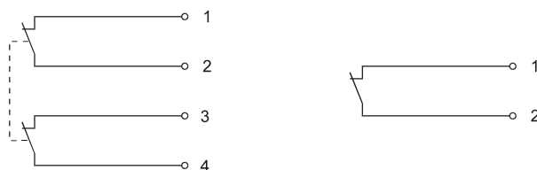
Figure A.7 – Connection of mechanical switches
