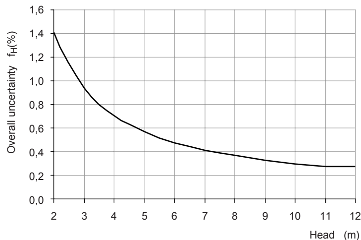
Figure 26 – Overall uncertainty of head for free water level for low head turbines
