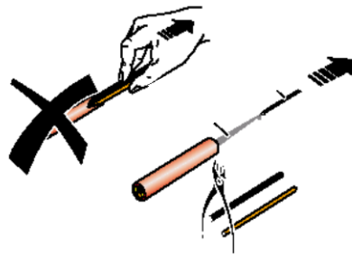
Figure 23 – Do not pull by the individual wires
