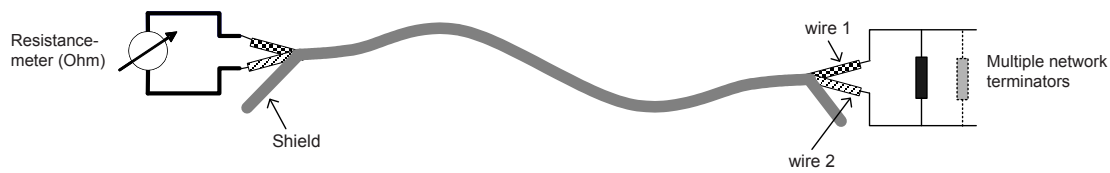
Figure N.5 – Resistance measurement between wire 1 and wire 2
