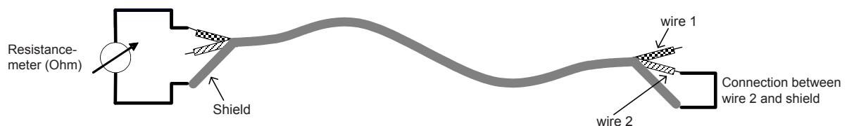
Figure N.4 – Resistance measurement for detecting wire shorts
