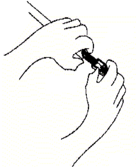
Figure I.4 – Inserting the cable into the connector body
