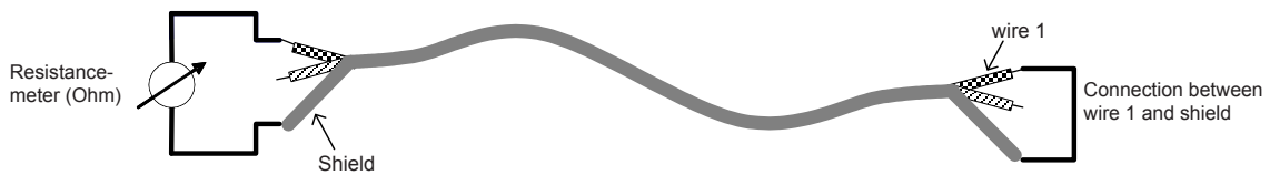
Figure N.2 – Loop resistance measurement wire 1 to shield
