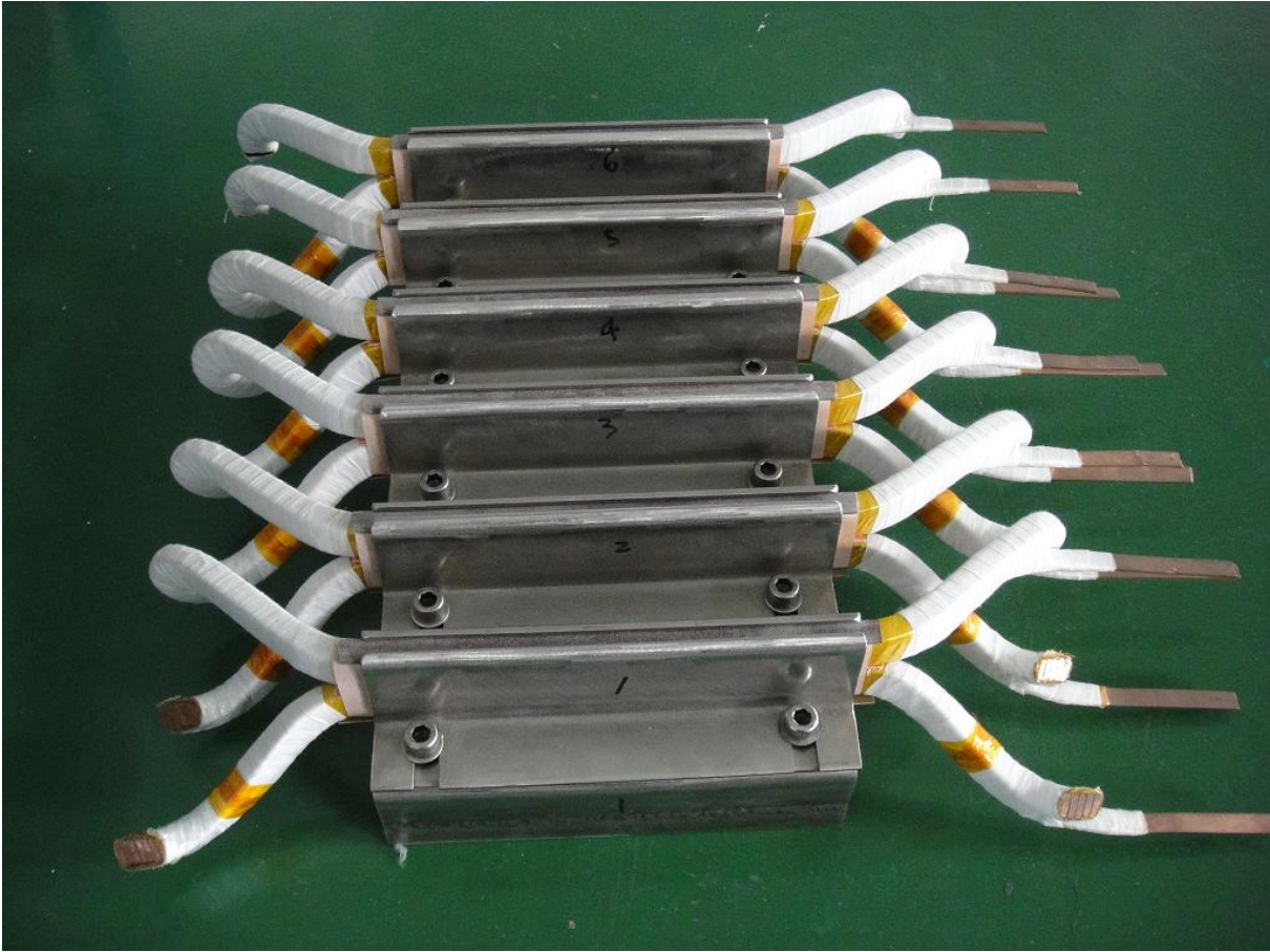
Figure B.8 – Formed coils placed into the form-wound test specimen or Formette
