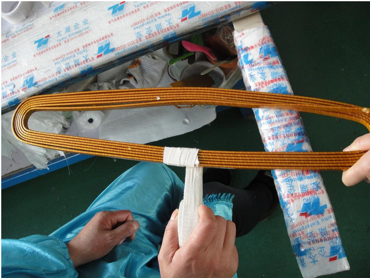
Figure B.2 – Un-formed coil being wrapped with a protective fabric
