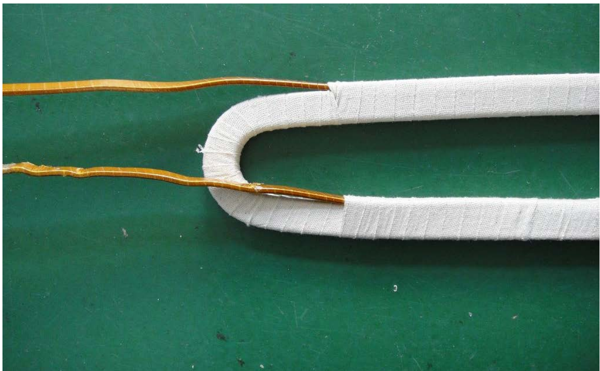
Figure B.2 – Un-formed coil being wrapped with a protective fabric
