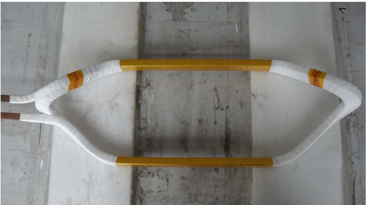
Figure B.6 – Close-up of formed coil's knuckle insulation
