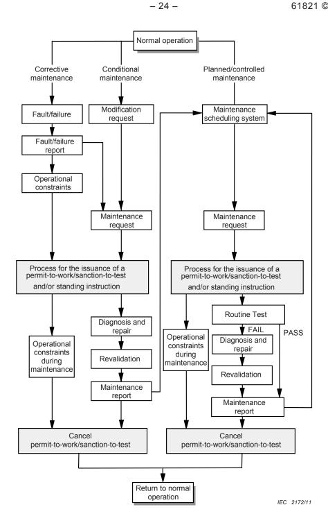
Figure A.2 – AGL constant current series circuit maintenance model
