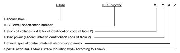
The coding of the monostable or bistable relay type shall be combined with the rated power of the coil, if applicable. The reference to two change-over contacts shall be given on the front page of the specification.
