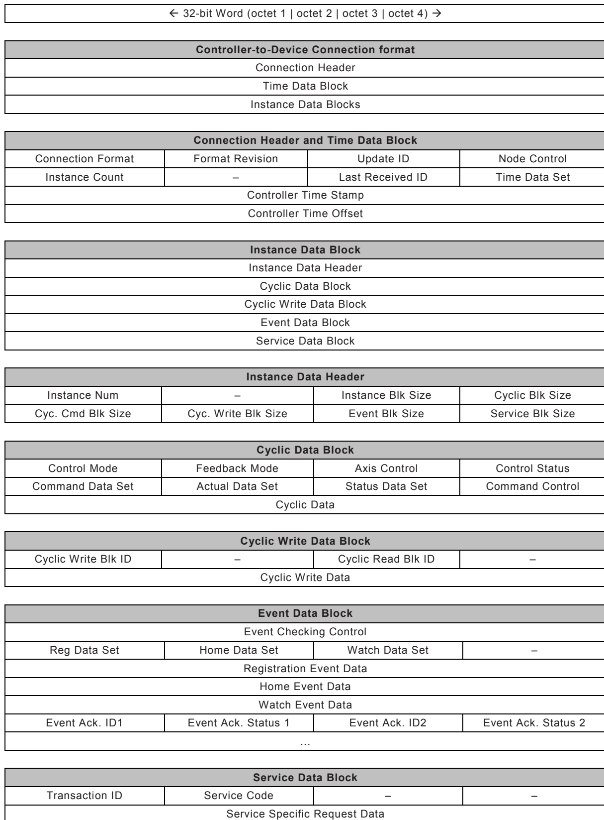
Figure 12 – Controller-to-Device Connection format (Connection Point 2)
