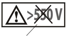
The pictogram and outline shall contrast with the background. The value of the voltage shown on the marking shall be 1,1 times the maximum phase to phase voltage.
