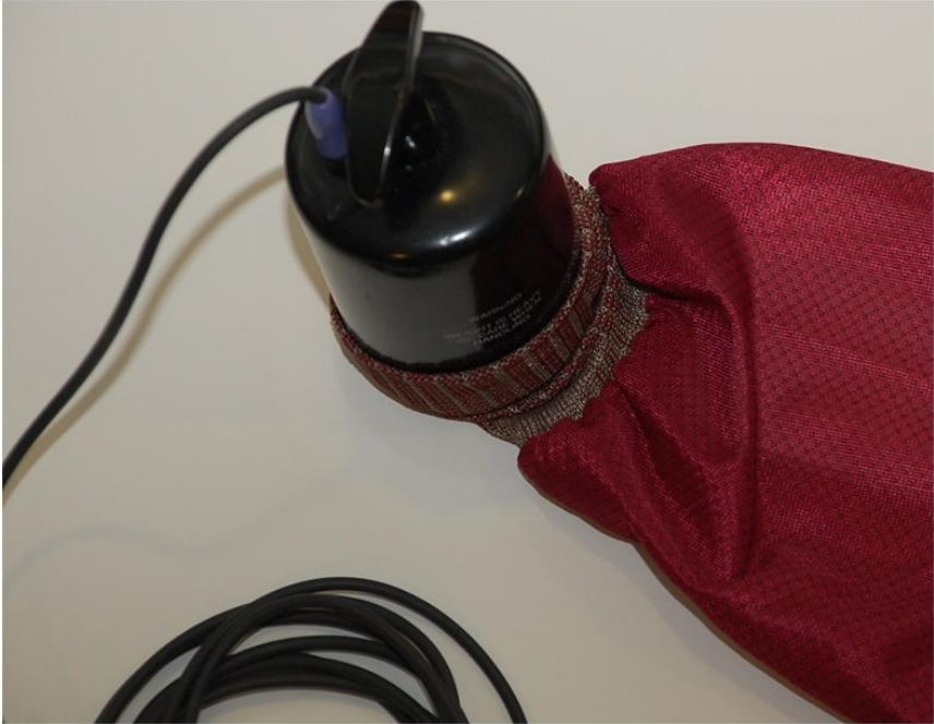
Figure 5 – Test set-up – Resistance point-to-point (electrode inserted into cuff detail)
