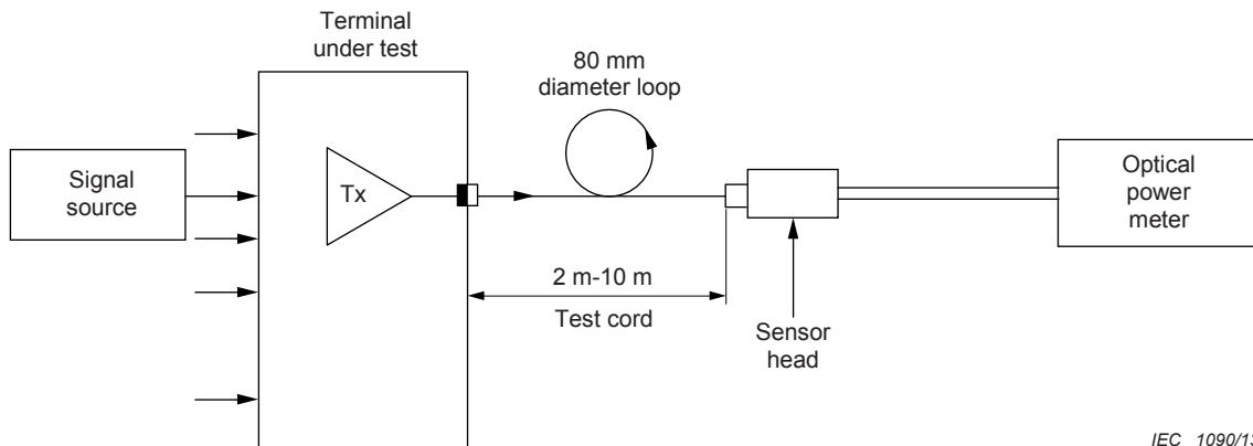
**Figure 1 – Transmitter output power measurement configuration**
