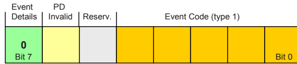
Figure A.22 – Structure of Status Code type 1
