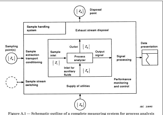
Figure A.1 — Schematic outline of a complete measuring system for process analysis consisting of a process analyzer and a sample handling system [6]
