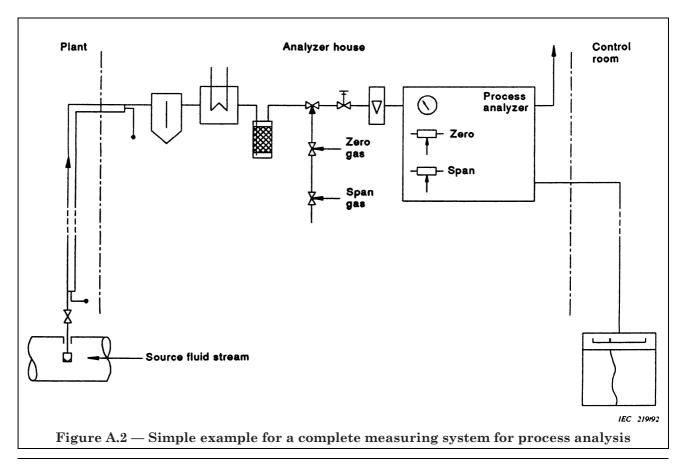
Not all of the basic functions have to be realized in all cases. "Sample stream switching", is comparatively seldom necessary, and for in-line or *in situ* analyzers the functions "sample extraction", "sample transport" and "sample conditioning" need not be performed, whereas the function "supply of utilities" may nevertheless be needed. For some portable and battery driven analyzers (e.g. for workplace hygiene measurements) a sample handling system is not necessary.
