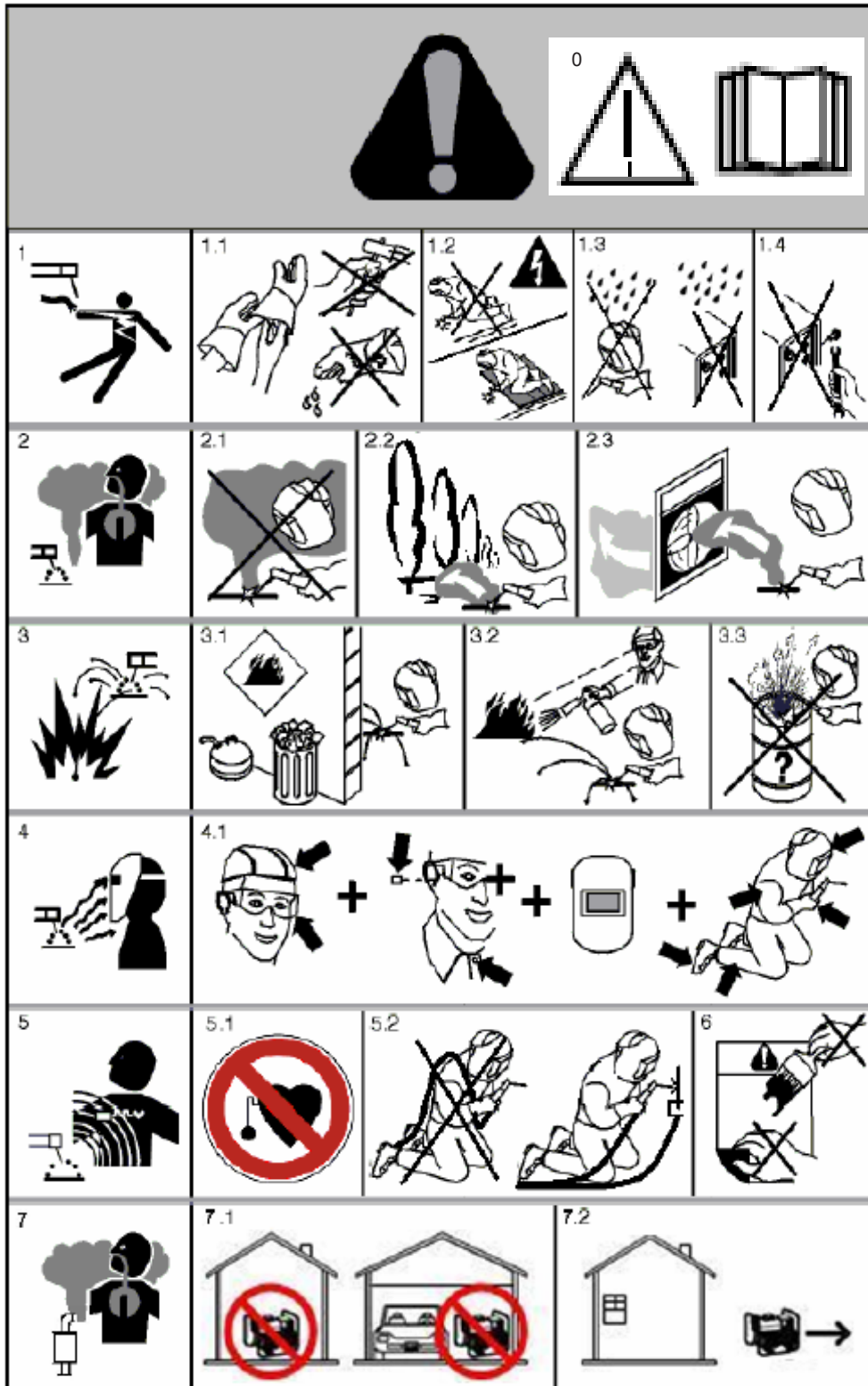
Figure C.1 – Example of precautionary label for engine driven manual metal arc welding power source
