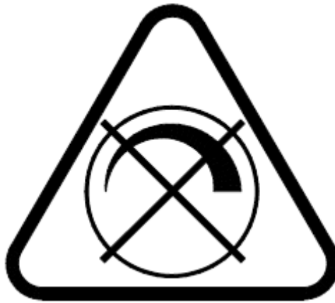
Figure 1 – Dimming not allowed
