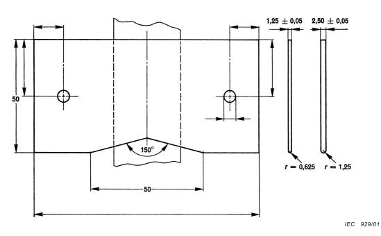
Figure 1 – Edge-tearing stirrup
