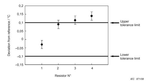
NOTE At each test result the expanded uncertainty (k=2) is indicated. Measurement uncertainty of manufacturer and user are assumed to be the same.
