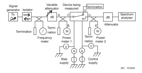
NOTE 1 Connect the point C to the input port, the point D to one of the output ports, and the point G to the other output port of the device being measured.
