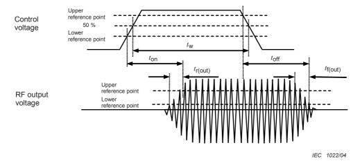
$\land$  NOTE  $t_w$ : Average pulse duration. Determined as the pulse duration at 50 % relative pulse amplitude of the control voltage.  $\land$
