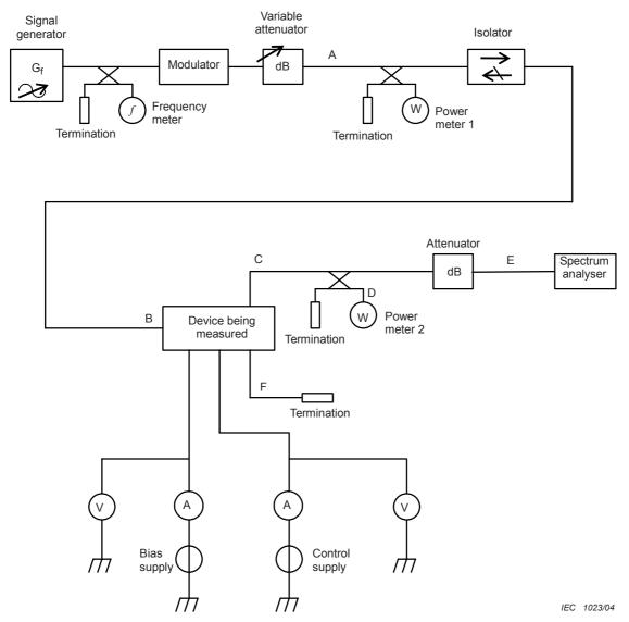
NOTE 1 Connect point B to the input port, point C to one of the output ports, and point F to the other output port of the device being measured.
