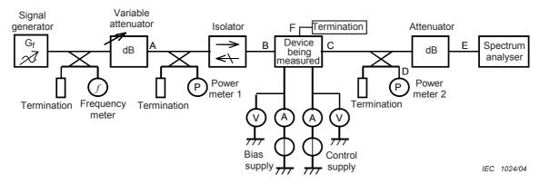
NOTE 1 Connect point B to the input port, point C to one of the output ports, and point F to the other output port of the device being measured.
