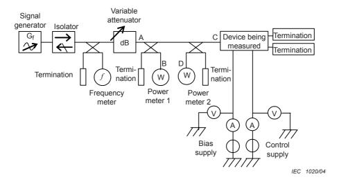
NOTE 1 Connect point C to the port to be measured and terminate the other ports of the device being measured.
