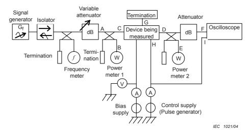
NOTE 1 Connect point C to the input port, point D to one of the output ports, and point G to the other output port of the device being measured.
