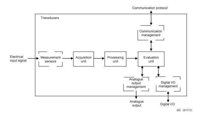
Figure 1 - Transducer architecture
