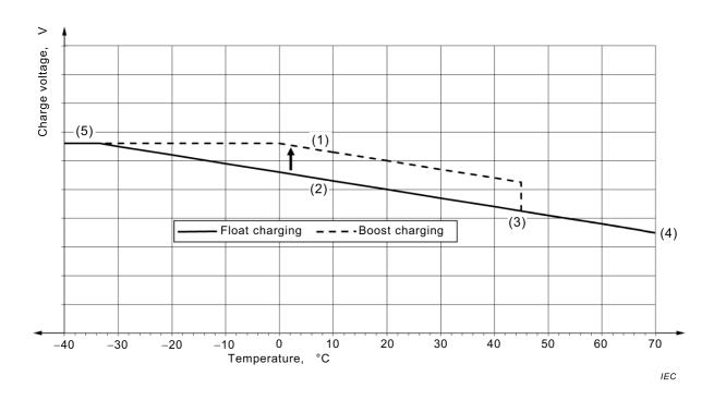
NOTE This figure shows a temperature compensated charging of -3 mV/ °C per cell based on 20 °C for Ni-Cd technologies batteries constant voltage charging (1 or 2 levels) with a current limit.
