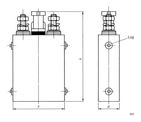
NOTE 1 Cells in steel container can have two or more terminals and four or more lugs.
