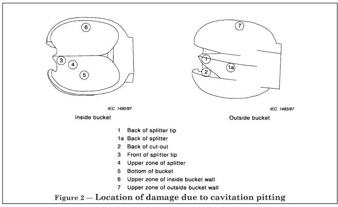
A second condition for the damaged area can also be the amount of damaged area  $A_i$  of an individual bucket, taking into account the non-uniformity/disparity in cavitation pitting from one bucket to another one. In this respect, the following will apply:
