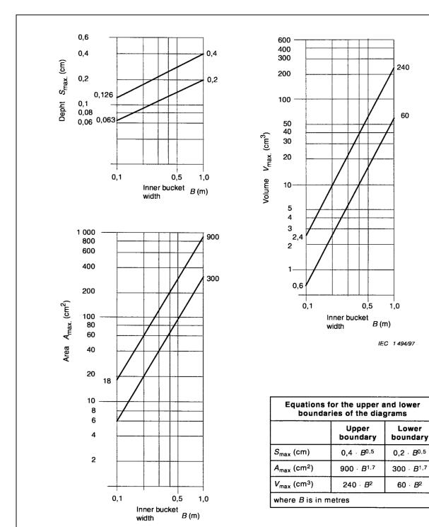
Figure A.1 — Examples of maximum permissible values of cavitation pitting on a Pelton runner (for the reference duration of 8 000 h)
