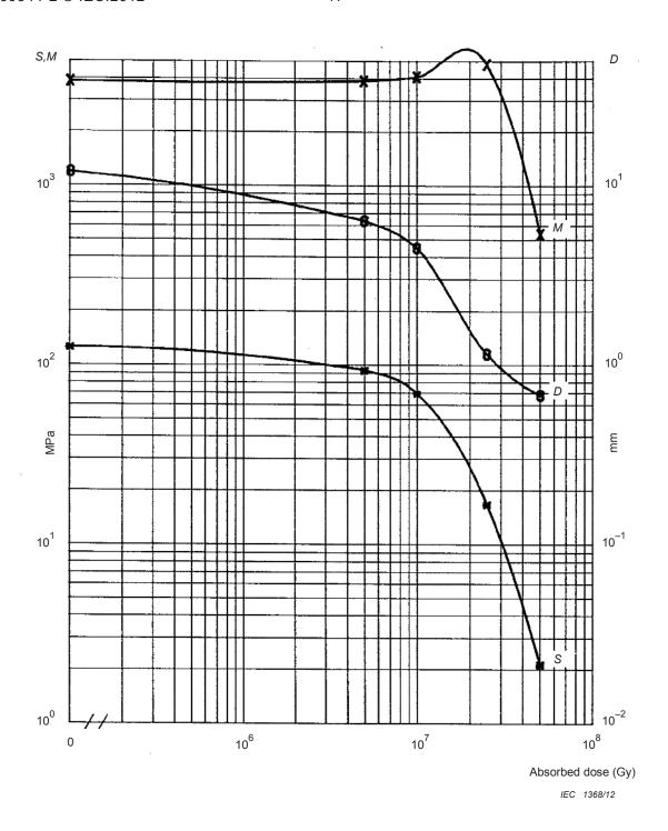
Figure A.1 – Change of mechanical properties as a function of absorbed dose for magnetic coil insulation
