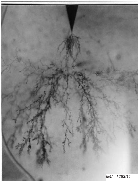
Figure A.26 – Electrical tree
