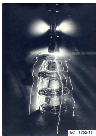
Figure A.16 – Corona on top and arcing to ground
