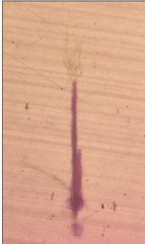
Figure A.36 – Water treeing
