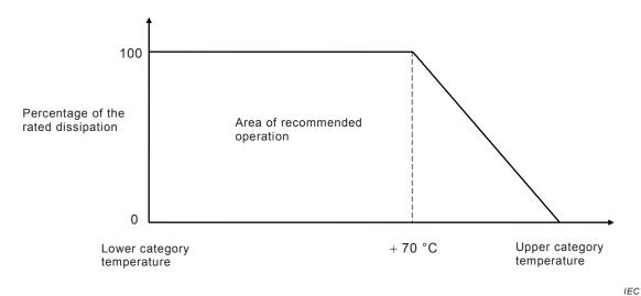
Figure 1 - Rated dissipation curve
