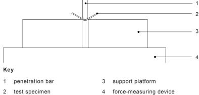
Figure 3 – Apparatus for measurement of stiffness
