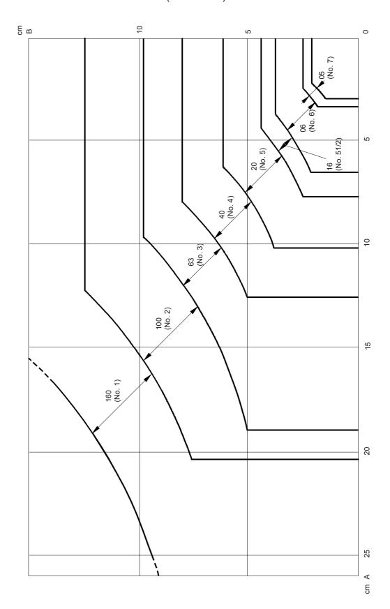
Figure A.1 – Grading chart for mica blocks, thins and splittings
