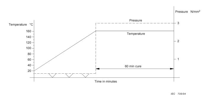
Figure 2 - Conditions for press procedure
