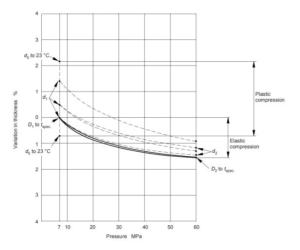
Figure 5 - Elastic compression, plastic compression
