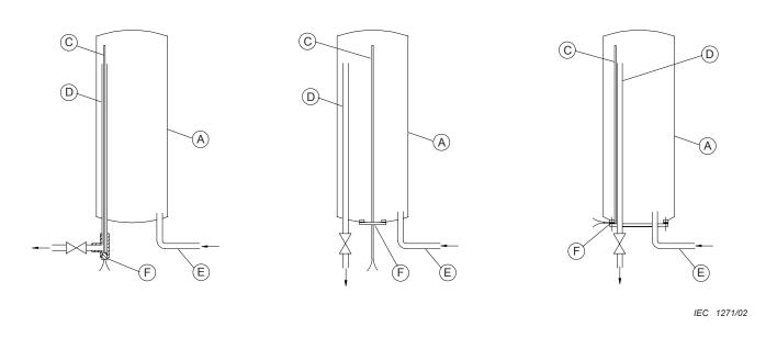
The thermocouple in a tube is inserted in the outlet pipe through a sealed entry
