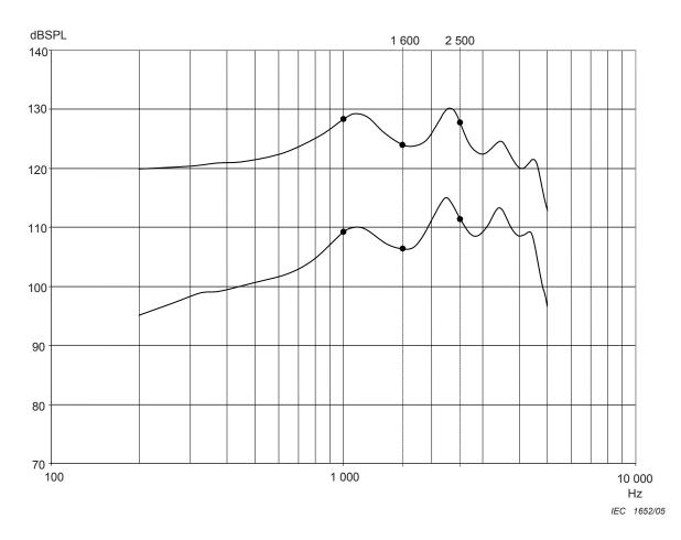
Figure 3 - Example of OSPL90 and basic frequency response curves
