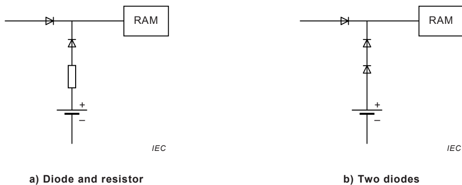
Figure 8 – Examples of safety wiring for charge protection
