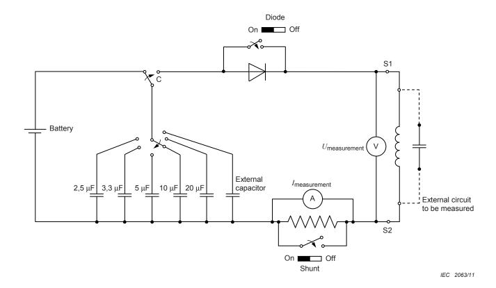
Figure A.5 – Example of measurement device
