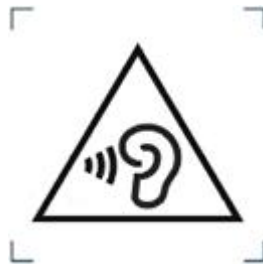
Figure Z1 – Warning label (IEC 60417-6044)
