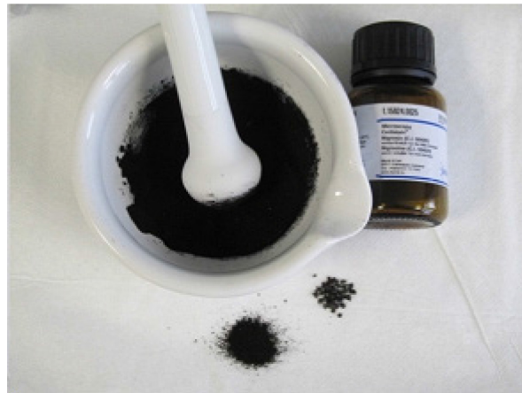
Figure 3 — Coarse Nigrosin kernels are ground in a chemical mortar
