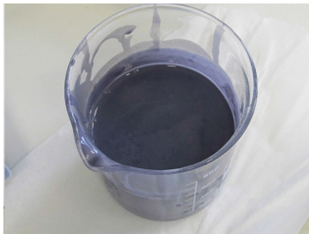
Figure 4 — Mixed test soil
