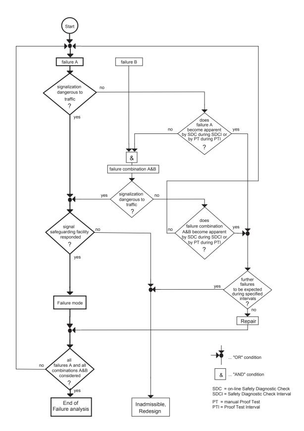
Figure 1 – Failure consideration of a Road Traffic Signal System – Protection against accidents caused by technical failures
