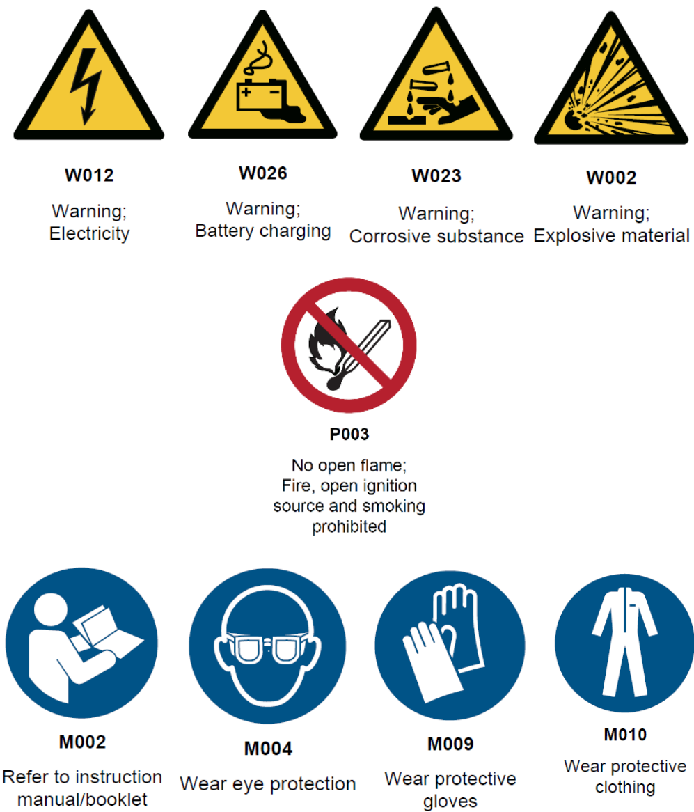
Figure 19 – Safety signs inside the battery box
