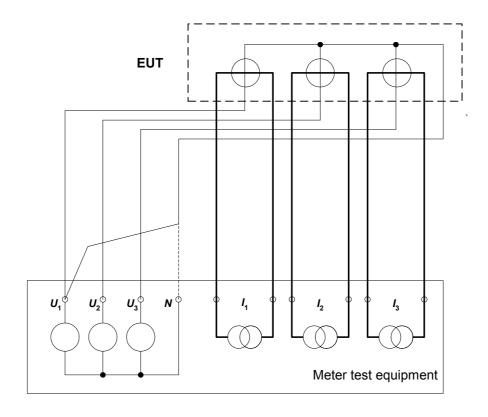
Figure B.1 – Circuit to simulate earth fault condition in phase 1
