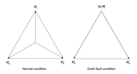
Figure B.2 - Voltages at the meter under test
