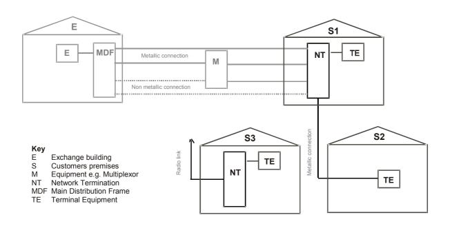
Figure 1 - Equipment with telecommunication ports installed at customers premises
