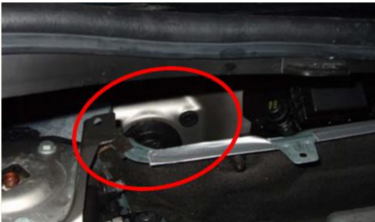
Figure D.1 — Location of ground installation point
