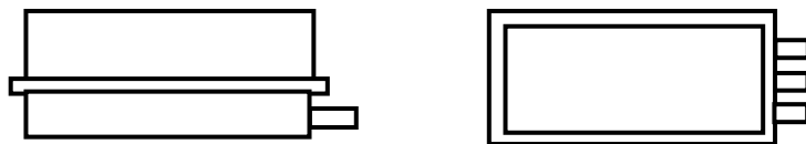
Figure 6 – Pan – Entry ports in one position at 90° to the rectangular cover removal axis
