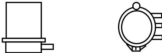
Figure 5 – Pan – Entry ports in one position at 90° to the circular cover removal axis
