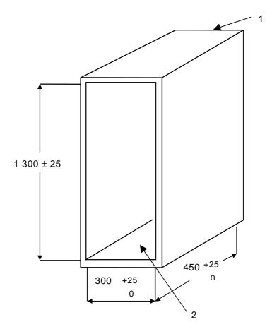
Dimensions in millimetres Material metal All measurements given inside
