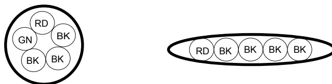
Figure 11 – Examples of cable or plug constructions where identification is done by configuration
