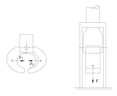
Figure 3 – Self-acting opening test – Tackle-points to strain the blade(s)
