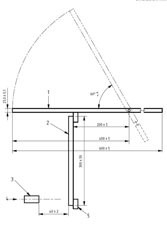
Key1shock producing device4centre line of burner face2test wall5support framework3gas burner
