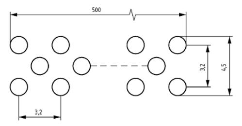
Round holes, 1,32 mm diameter, on centres 3,2 mm from one another, staggered in three rows and centred on face of the burner
