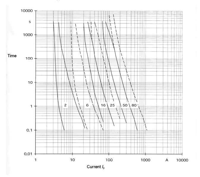
Figure C.1 — Fuse characteristic curve
