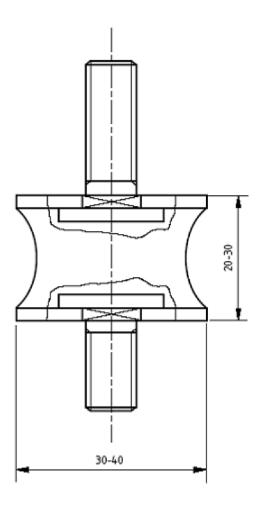
Figure 4 — Typical rubber bush (hardness: 50-60 shore A) for fastening the wall to the rigid supports
