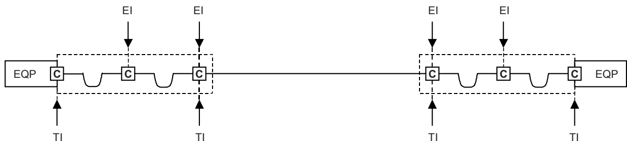
Figure 5 – Test and equipment interfaces for backbone cabling
