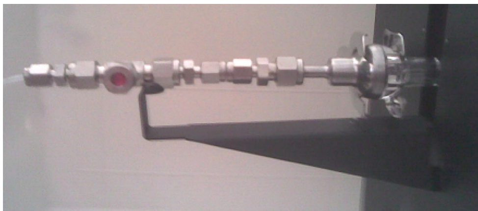
Figure B.1 — Inserting a T with a septum to the carrier gas line of a Sunset lab carbon analyser
