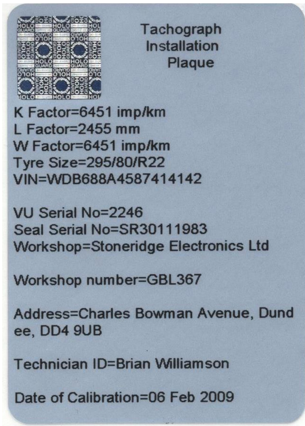
Figure B.2 — Second example for installation plaque
